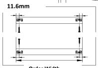
Match the outer edge of the Shoe Base to the marked position, and allocate a minimum distance (L1) from wall to the front of Shoe Base. Install the Base with 1pc 25mm screw.
