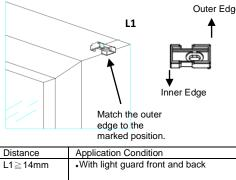
installing Shoe Bases at the ends, install two Bases in the center at top and one Base in the center at bottom, and keep them align with the end Bases. The outer edge of Bases should head to the middle line, as illustrated below. The bottom Shoe Base needs to align with the left one at the top center.
