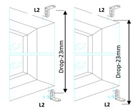
Top of the shade to the edge of bottom of the L bracket equals shade drop - 23mm
